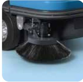
The side brush retracts in the event of accidental knocks, thus avoiding all possible damage. The brush's slanting angle can be adjusted to better adapt to cleaning along borders, etc.
