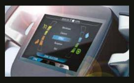
To ensure the desired cleaning results in all conditions and prevent the risk of tampering, the site supervisor can save a number of separate configurations with specific cleaning parameters for different work environments. The operator simply has to select the zone to be cleaned, and the machine is configured automatically with all the right settings
