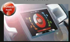
When more scrubbing power is needed, activating Power Mode increases the delivery rate of detergent solution and boosts brush pressure and vacuum power for the time necessary to tackle heavy duty cleaning
